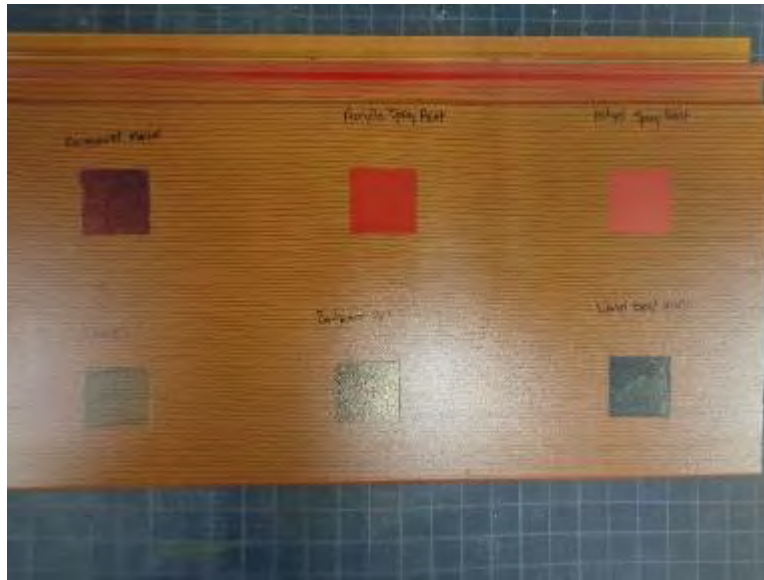
Photo No. 3 Panel with Graffiti
